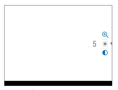
**Brightness** – press the **UP (4)** / **DOWN (2)** buttons to change display brightness from 0 to 20.
