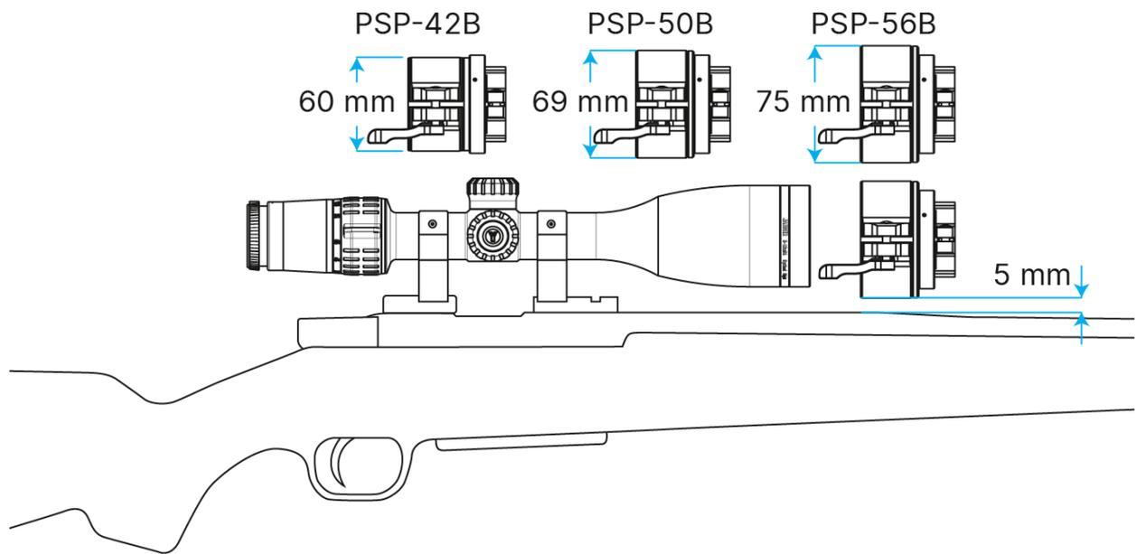
When installing the PSP B Ring Adapter on the riflescope, the gap between the adapter and the rifle body must be at least 5 mm.
