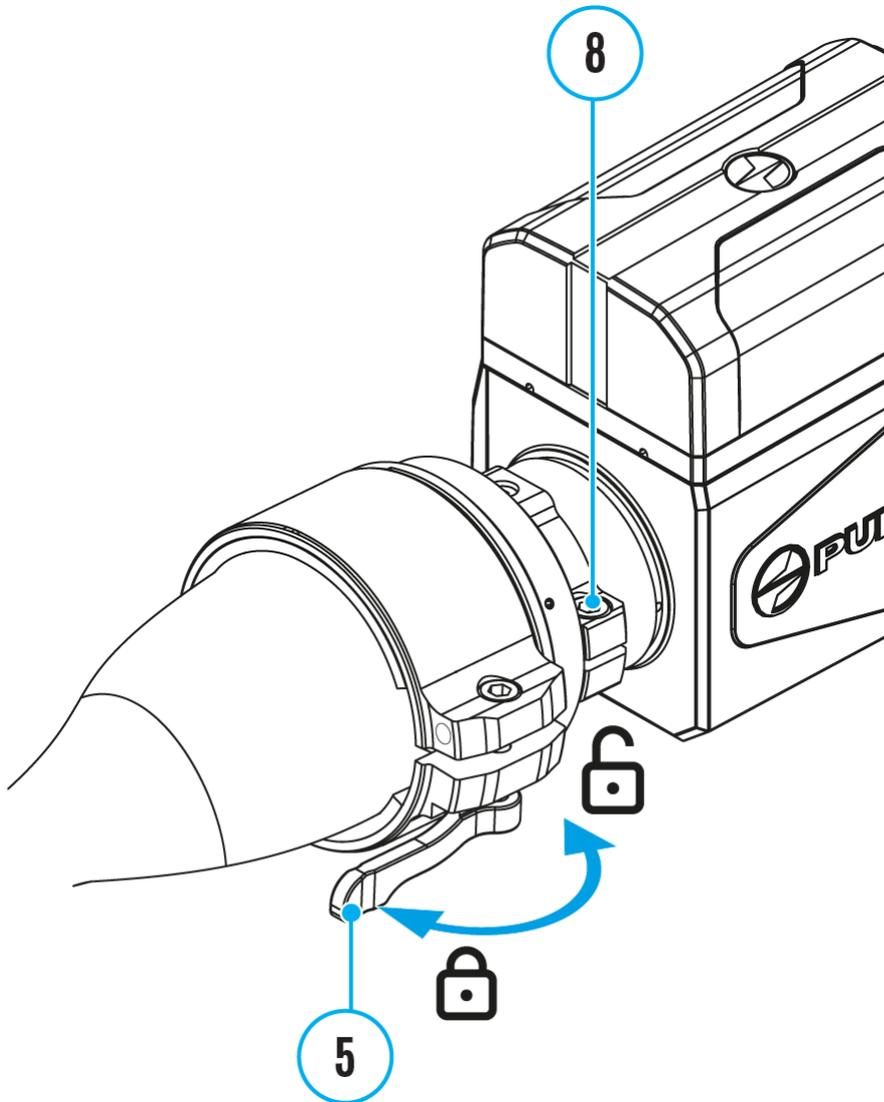
1. Loosen the screw **(8)** with an Allen key (S = 4mm).
