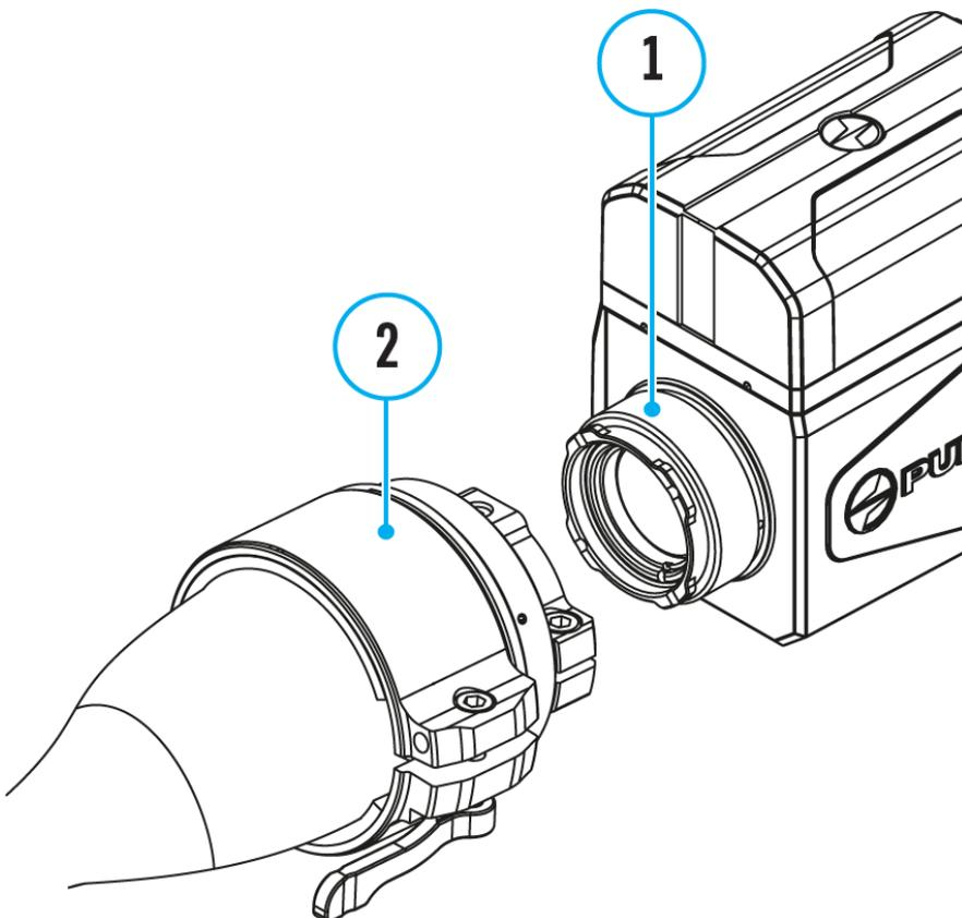
1. Remove the protective cover from the eyepiece of the thermal imaging module.
