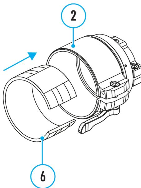
1. Apply 2-3 strips of double-sided tape to the outer surface of the insert of your choice **(6)**.
