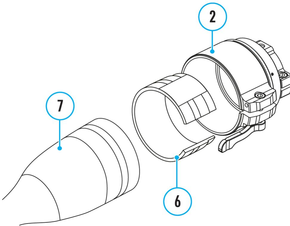
1. Select the Ring Adapter **(2)** with the insert **(6)** of the desired diameter depending on the outer diameter of the lens of your optical device **(7)**.
