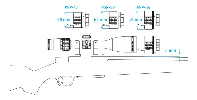
When installing the PSP Ring Adapter on the riflescope, the gap between the adapter and the rifle body must be at least 5 mm.
