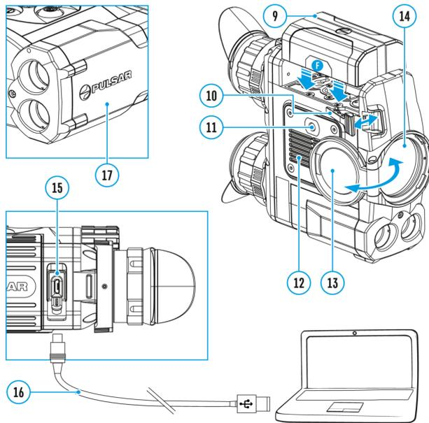
**Accolade 2 LRF Pro** thermal imaging binoculars feature video recording and photography of the image being ranged to the internal memory card.
