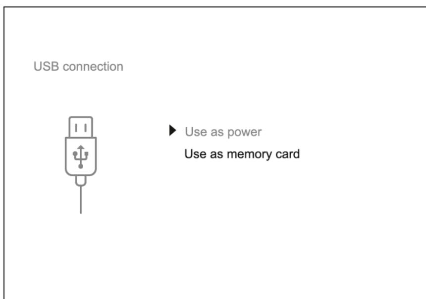
1. Connect one end of the USB cable **(16)** to the Micro-USB **(15)** port of your device, and the other end to the USB port of your PC/laptop.
