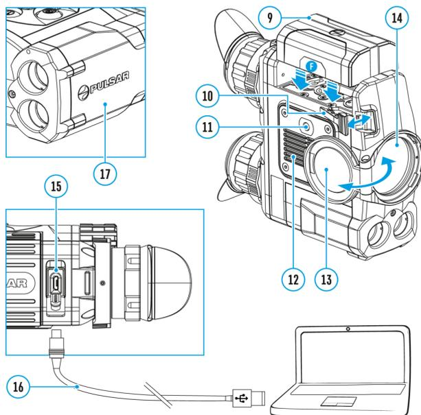
The device can be powered with an external power supply such as Power Bank (5 V).
