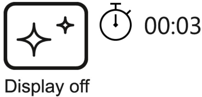
1. When the device is on, hold down the **ON/OFF (1)** button. Display goes out, message **"Display off"** appears.
