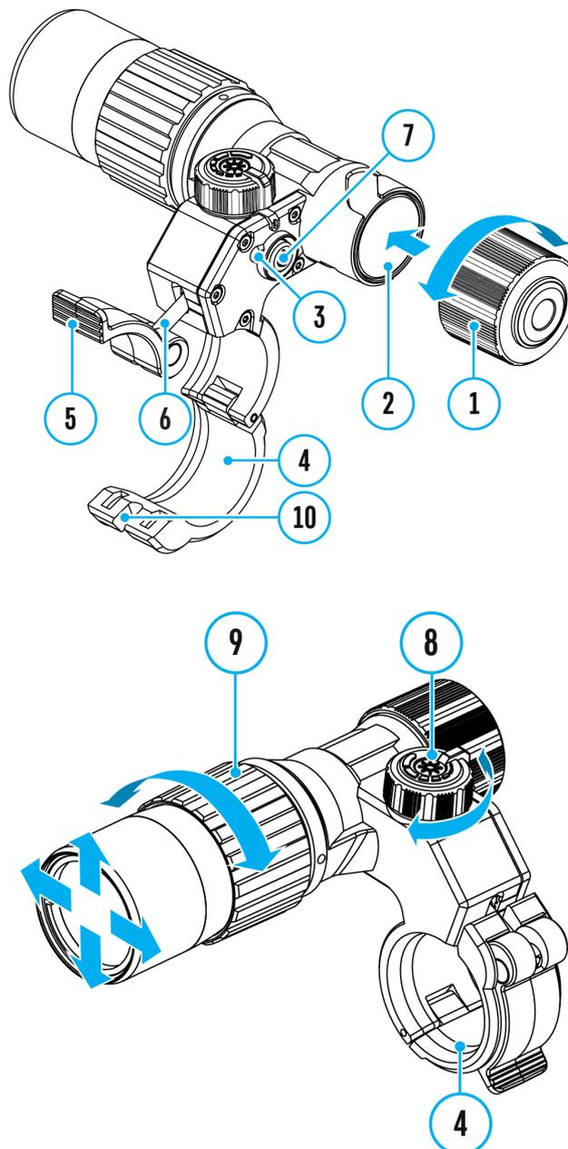
1. Turn on the IR illuminator by pressing the button **(7)** on the side of the illuminator housing.
