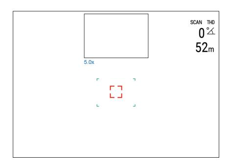
2. To exit SCAN mode, press LRF (6) button again.
