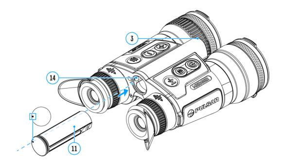
**Attention!** Before installing the battery, make sure that there is an undamaged rubber insulating ring on the battery. The ring is designed to protect your device from moisture getting inside. Damage to the device due to a missing ring is not covered by the warranty. To replace or purchase a ring, contact your **local distributor**.
