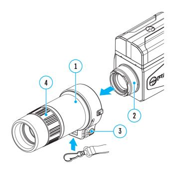
**1.** Align the protrusions on the monocular **(1)** on the side of its lens with the grooves of the mount **(2)** of the thermal imaging module.
