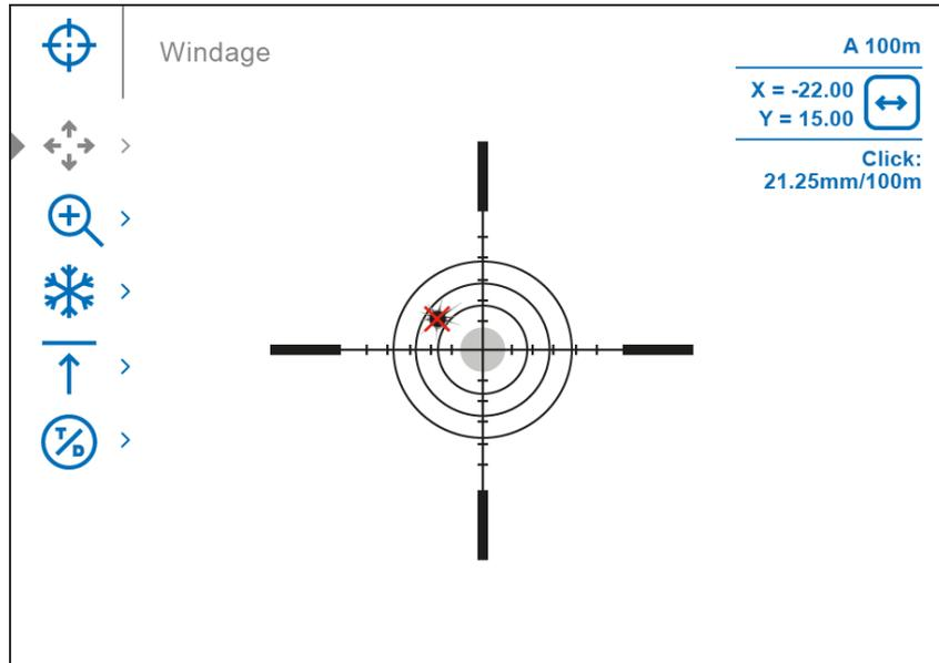
**6.** To change the direction of the auxiliary cross movement from horizontal to vertical, press the controller button **(6)** briefly.
