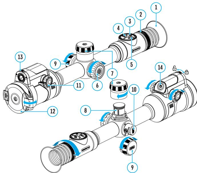
1. Press and hold the controller button **(6)** to enter the main menu.
