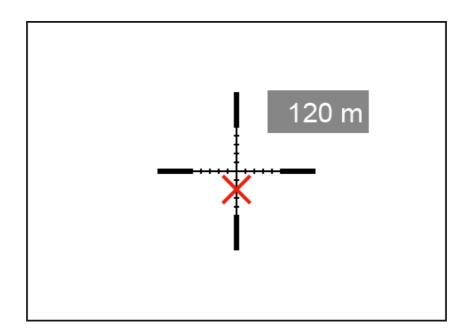
1. Rotate the controller ring (6) to select Auxiliary indication of distance
