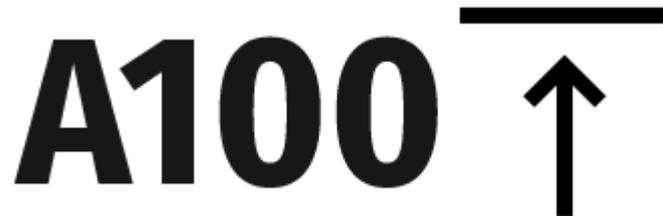
– information on the current profile and zeroing distance in this profile (e.g., profile A, zeroing distance of 100 m). This information is always displayed in the status bar. Rotate the controller ring **(6)** to switch between the zeroing distances in the selected profile. This function is available if there are two or more distances in the profile.
