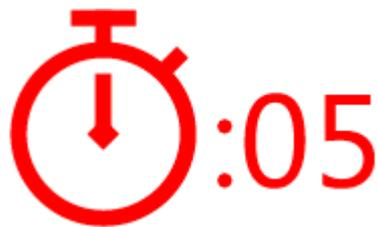
will appear instead of the calibration icon when in automatic calibration mode with 5 seconds remaining until automatic calibration; displayed only in thermal imaging mode and Multispectral PiP)
