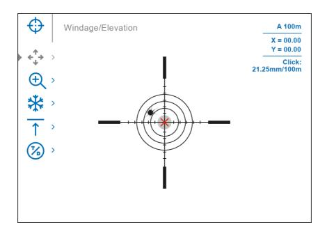
4. Press the controller button (6) briefly to enter the Windage/Elevation
