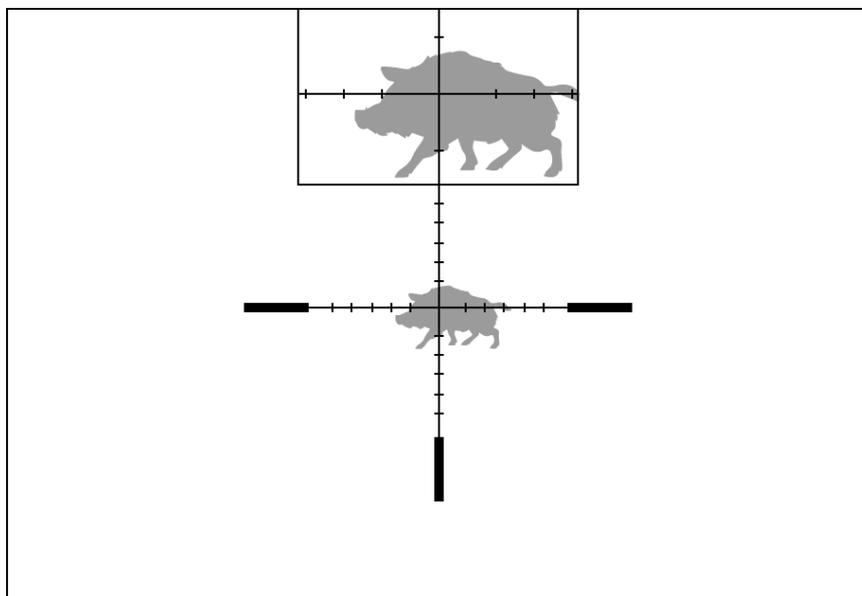
1. Press and hold the **ZOOM (5)** button to turn on/off the PiP function.
