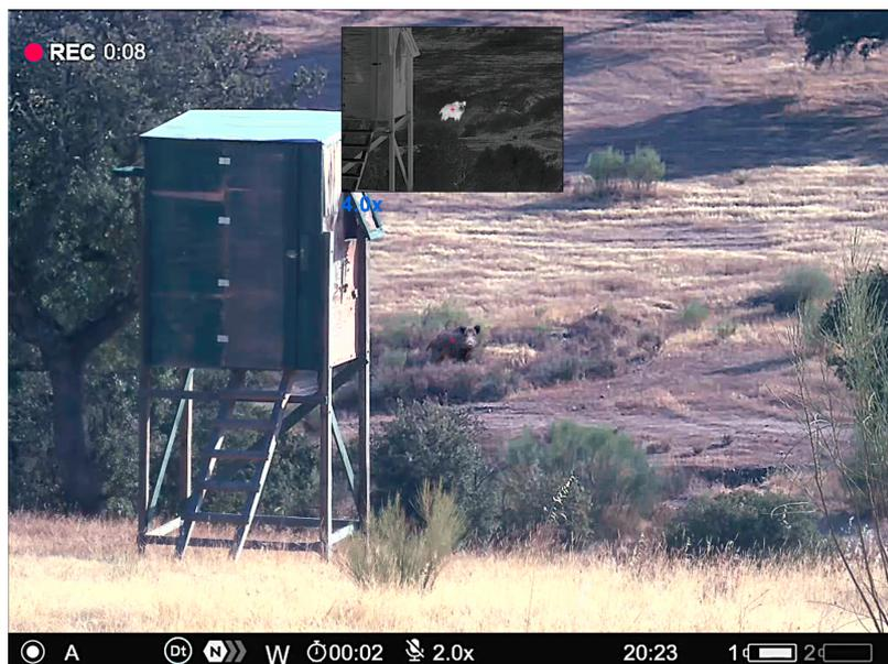
In the multispectral PiP mode, the image of one channel is displayed in the main window, and the image of the second channel is displayed in the PiP window.
