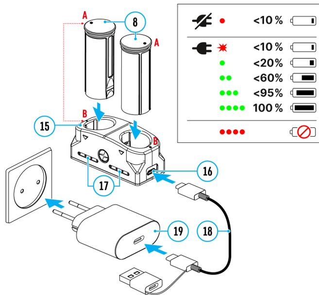
1. Insert the Battery Pack **(8)** along the rail into the APS charger **(15)** slot as far as it will go. The APS charger is supplied with your device or purchased separately.
