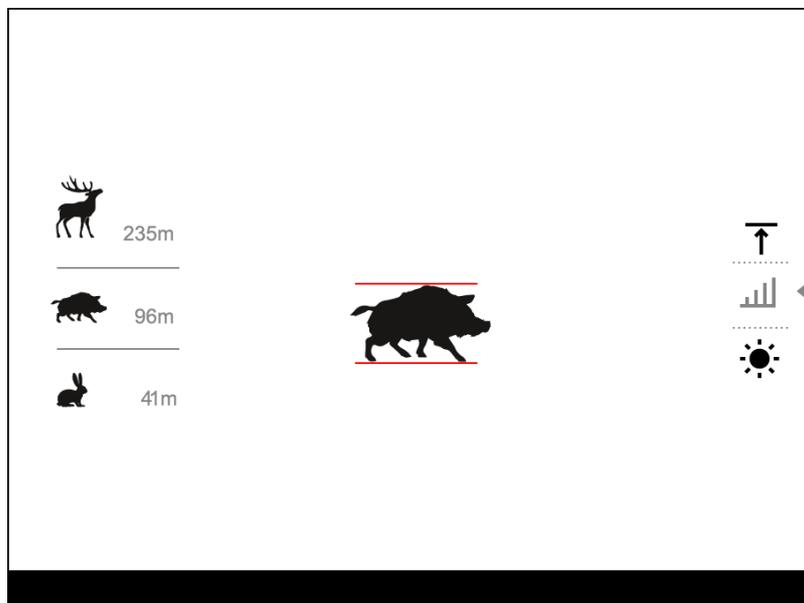
1. To select the **Stadiametric Rangefinder** function, enter the **Quick Menu** by briefly pressing the controller button **(6)**.
