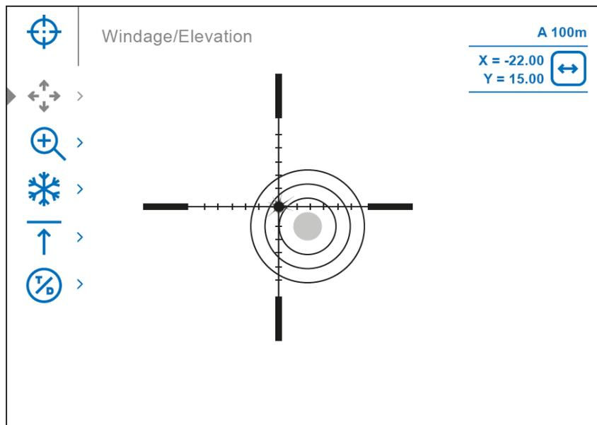
3. The coordinates for the digital and thermal channels will be saved under the same distance name. Zeroed channels are displayed in the status bar with icons
