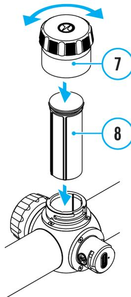
1. Turn the battery cover **(7)** counter clockwise and remove.
