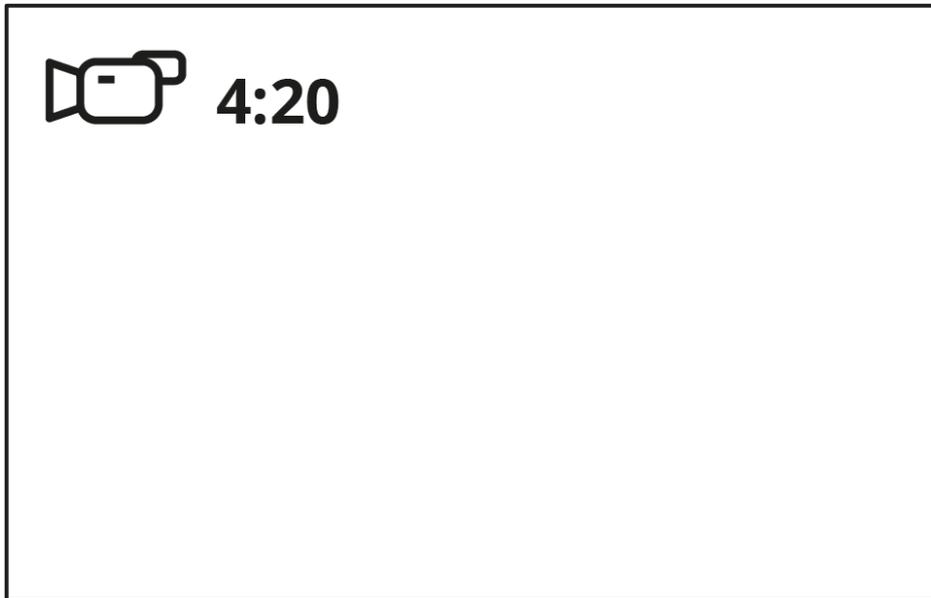
Toggle (switch) between the riflescope operating modes with a long press of the **REC (4)** button. Switching between the modes is cyclical (**Video**→**Photo**→**Video**...).
