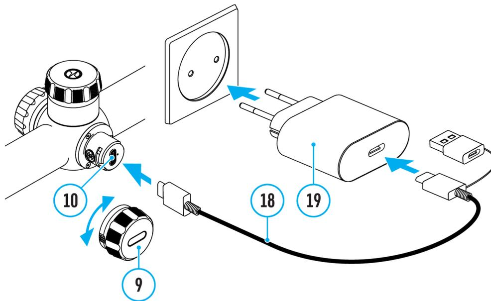
1. Open the USB Type-C cover **(9)** by turning it counterclockwise.
