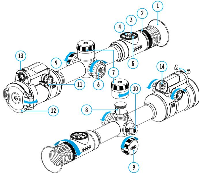
1. Open the thermal channel lens cover **(12)**.
