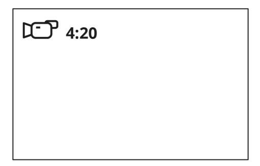
Toggle (switch) between the riflescope operating modes with a long press of the **REC** (4) button. Switching between the modes is cyclical ( $Video \rightarrow Photo \rightarrow Video...$ ).
