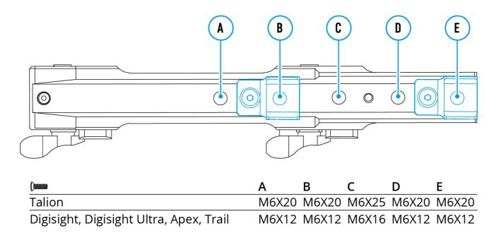
• To install the mount on Digisight/Digisight Ultra, Apex, Trail riflescopes, disconnect the adapters **(6)** using an S2.5 Allen key.
