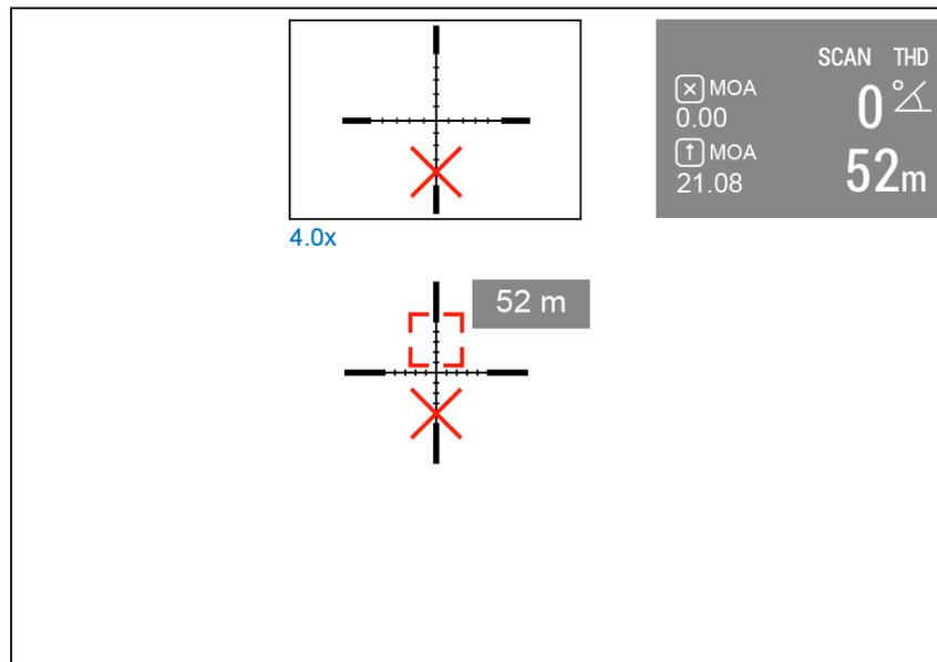
12. To manually adjust the SPOA of the ballistic calculator, select the desired distance in the quick menu:
